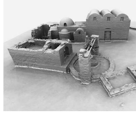
3D model of the site derived from a laser scan survey
