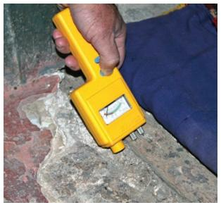
FIGURE 71 Very high moisture levels could be recorded underneath the carpet in the Sanctuary
