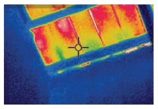
FIGURE 29 Infrared image of the top of the south wall. Note that the moisture content of the wall (blue) is quite even
