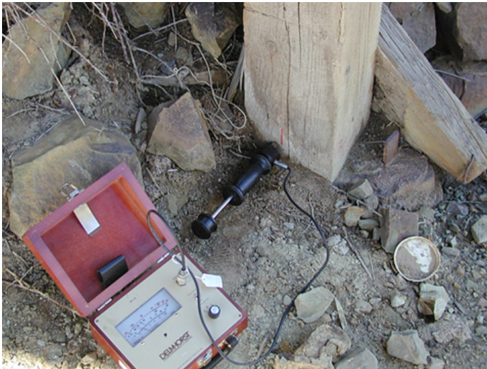
Figure 12. Conductance-type moisture meter being used on a timber post in ground contact.
